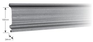
0.8mm, continuous roll formed, interlocking, coated galvanised steel slats. Nominal effective pitch of 100mm. Zinc coating of not less than 275g/m<sup>2</sup>.
