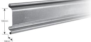
1.0mm, continuous roll formed, interlocking, coated galvanised steel slats. Nominal effective pitch of 100mm. Zinc coating of not less than 275g/m<sup>2</sup>.
