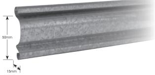
0.8mm, continuous roll formed, interlocking, coated galvanised steel slats. Nominal effective pitch of 50mm. Zinc coating of not less than 275g/ m<sup>2</sup>. The curtain is fitted with moulded nylon clips to the ends of alternate slats by two nylon rivets.
