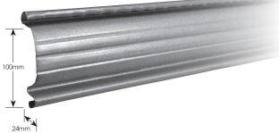
High tensile G550 continuous roll formed, interlocking, coated Galvabond® steel slats. Nominal effective pitch of 100mm with 3 small ribs. Zincalume® coating of not less than 150g/m<sup>2</sup>. Moulded nylon clips fitted to end of alternate slats by means of three nylon rivets.
