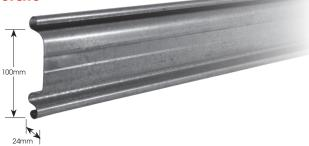
0.6mm, continuous roll formed, interlocking, coated galvanised steel slats. Nominal effective pitch of 100mm. Zinc coating of not less than 275g/m<sup>2</sup>.
