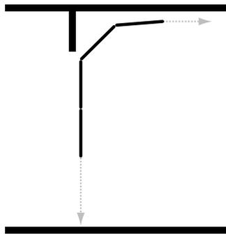
**Sectional doors** – comprise of a number of rigid sections that are hinged together and move vertically in the opening, then horizontally along the ceiling, guided by tracks and counter-balanced with springs. Commonly used on new houses where a pattern or style is required to match the style of the house. These doors can be made of steel, wood and other materials. The B&D Panelift® range offers a broad selection of styles and colours.
