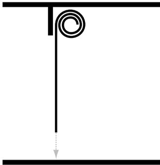
**Roller doors** – comprise of a ribbed steel curtain that moves vertically in the opening, and rolls up around a drum, guided by tracks and counterbalanced with springs. They are particularly suitable for garages and sheds where there is plenty of headroom above the opening and where a traditional look is required. The B&D Roll-A-Door® is the original roller door, with 50 years of added innovation and improvement.
