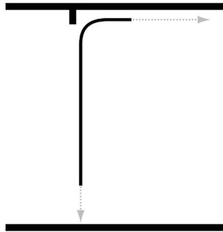
**Flex-A-Door® doors** – comprise of a durable Roll-A-Door® curtain, fitted on a curving track, which slides from a vertical position up into a horizontal position, close to the ceiling. Especially suited to applications where there is not the headroom for a roller door or, where a smoother, easier to use solution is required to replace an existing tilt door.
