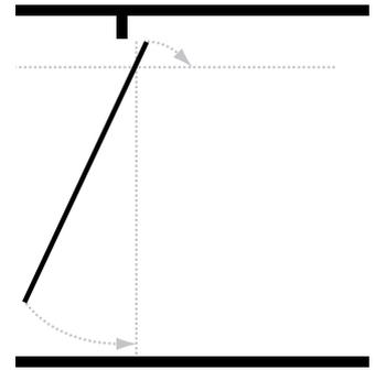
**Tilt doors** – comprise of a one piece tilting panel, fitted with pivoting arms at both sides of the opening, which moves out and up from a vertical position into a horizontal position. These allow almost any material to be used to make a garage door and offer one of the lowest possible headroom requirements. When you choose B&D Tilt-A-Dor® fittings, you can be sure quality hardware is included in your tilting door.
